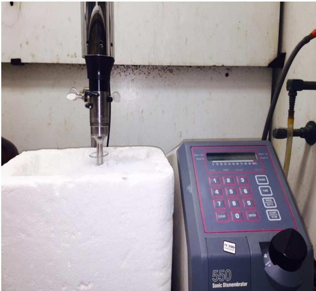
Figure 9 Ultrasonication of PCPU + nanoparticles
